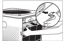
3. Remove dust with water or a vacuum cleaner depending on the degree of contamination.
